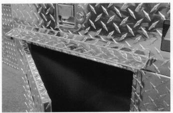
Center the 19" rain gutter above the dog compartment door. Make sure the rain gutter does not obstruct the door from opening before drilling. See illustration above. Follow steps 3-5 to complete the installation. Use the same procedure for the other dog compartment door.
