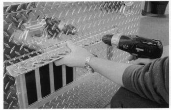
Using the pre-punched holes in the rain gutter as a guide, drill a 3/16" hole through the aluminum wall of the dog box. See illustration above.
