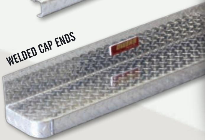
Aluminum boards are constructed of .100 diamond tread with a 4" riser for heavy use and are offered with your choice of either welded end caps or bolt on stone guards and end caps.
