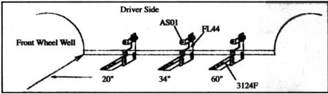
3. Measure from front wheel well, back 20", 34" and 60". Mark these bracket locations. Note: Steel plates have been inserted under fiberglass to mount brackets securely using self-drilling screws. Double check your marks to be sure they line up with the steel plates before drilling.
