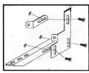
4. Assemble bracket components with 5/16" nuts & bolts as shown. Do not tighten at this time.
