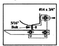
5. Drill 5/16" hole in pinch weld so that AS01 on bracket assembly mates at pinch weld. Secure with 5/16" nut and bolt, then install #14 x 3/4" self-drilling screw at top of FL44.
