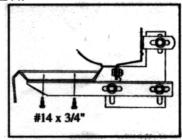
Screw step to bracket using two #14 x 3/4" self-drilling screws per bracket.
