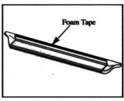
Apply foam tape to top edge of GlaStep. Remove protective strip from top edge of foam tape.
