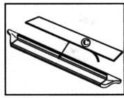
9. Place pad on step. Peel off tape backing to secure. Don't forget the Owens label!
